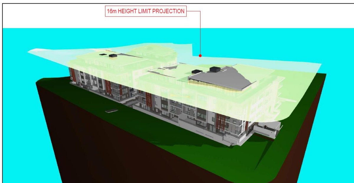
Figure 18: Extract of Height Plane from DA 20/2016/JP from the former Hills Shire Council showing extent of non-compliance with 16 metre building height.
