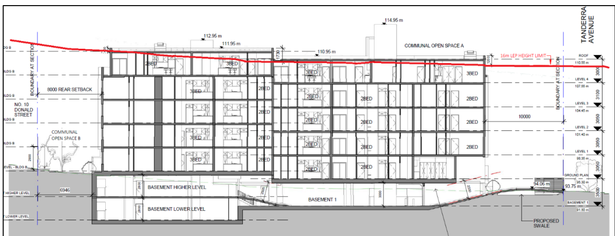
Figure 16: Extract of Section AA showing exceedance in building height.
