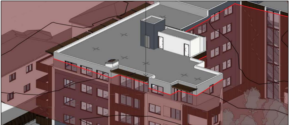
Figure 15: Enlarged extract of Height Plane. Where the height plane crosses through the building has been indicated by the red line.
